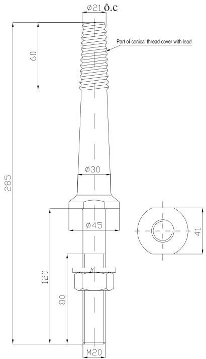
TY SỨ ĐỨNG 24 KV(BOC CHI) PIN OF 24KV PIN INSULATORS
